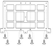
3. Match the position of installation bracket and installation plate with screw A.
